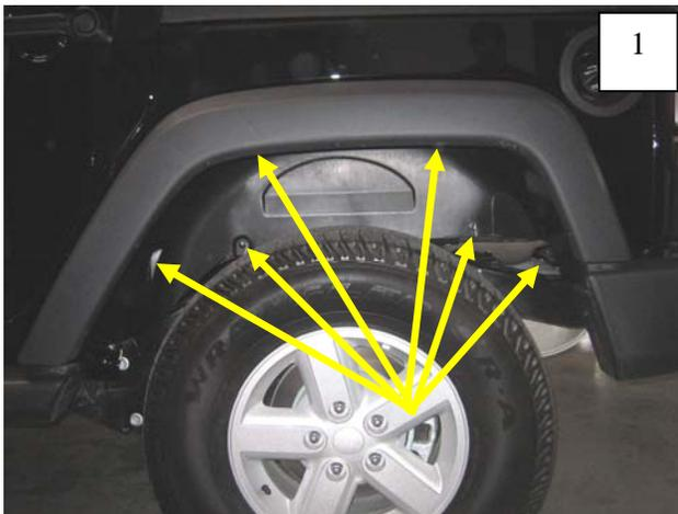
Using a pry tool, pliers, or a flat head screwdriver, remove six plastic fasteners from inside of splash shield.
