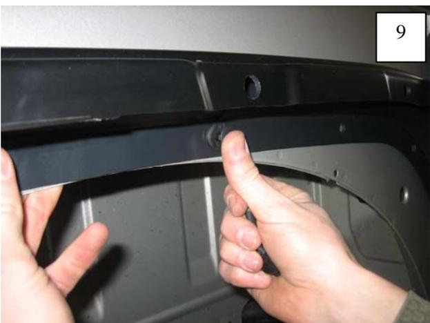
Position Inner Flare Piece on fender, aligning existing 5/16" holes in Inner Flare Piece with holes in fender. Install supplied Plastic Push Retainers (9 places).
