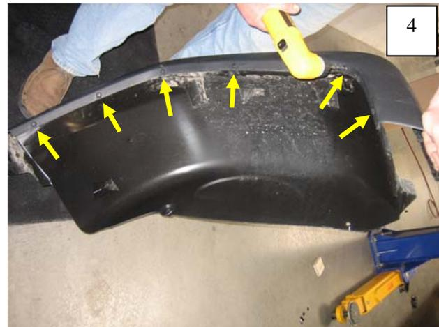
Use a drill with a 5/16" bit to drill through six plastic rivets along edge of flare/splash shield. Discard the flare, but retain the splash shield. **NOTE:** It is helpful to angle the drill while drilling the rivets.
