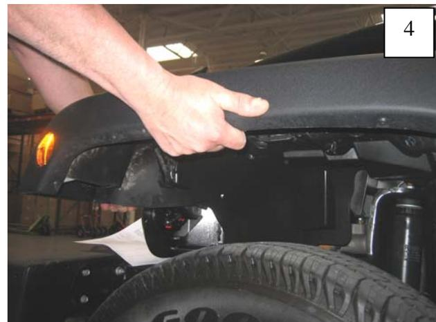
Starting at front of flare, pull firmly to release flare and splash shield from fender, working your way to the back. You will hear popping noises as clips release. It is O.K. if clips break, they will be discarded.
