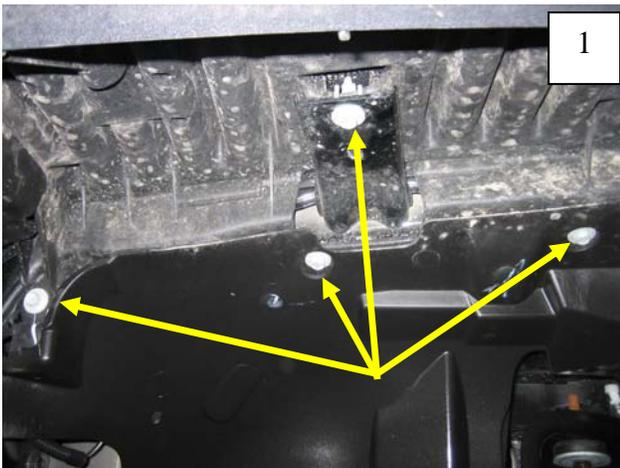
Using a socket wrench with a 10mm socket, remove four factory bolts from inside of splash shield. Retain all bolts.
