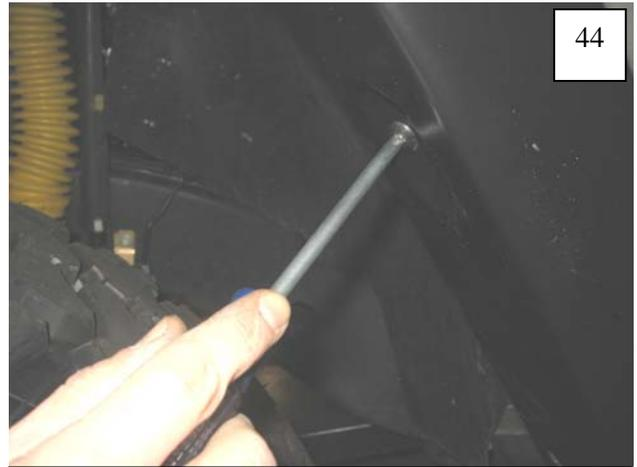
Install supplied Truss Head Screws through holes in wheel well and into #14 U-Clips installed in Step 25 (6 places). Ensure proper alignment of outer flare, inner flare, and splash shield. **Do not tighten.**
