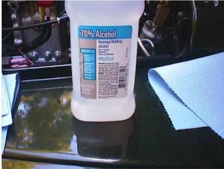
Clean each door top one more time (fourth time). This time dry the alcohol off with a clean dry paper towel. If you see any dirt/wax film streaks while doing this repeat the cleaning process until spotless.
