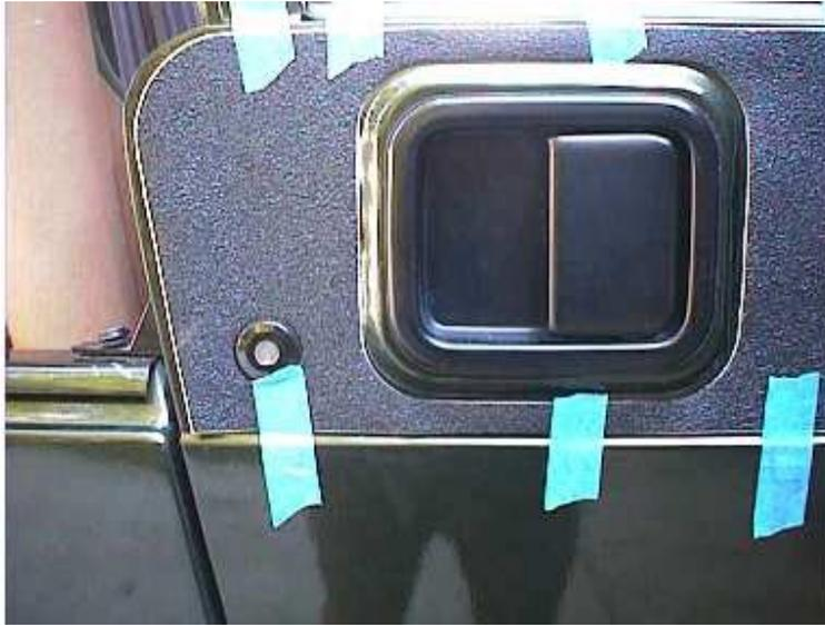
Securely tape the Door Protectors in the proper location using masking tape. Make sure there are no voids under the Protectors.
