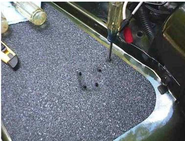
Enlarge these holes by rotating the screwdriver to their proper size.
