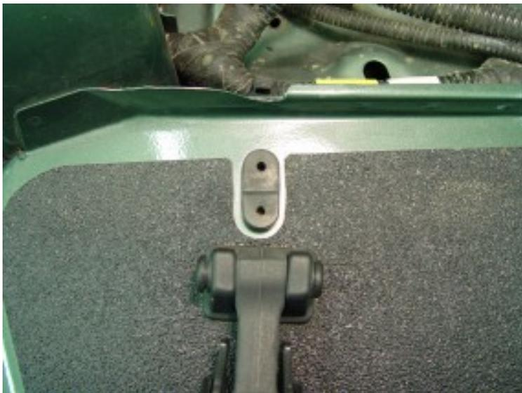
To install the Rubber Bumper first lubricate the two nipples with water or a window cleaning solution. Then insert a small screwdriver into the holes on the top of the rubber bumper and press it into place through the Protector and into the fender.
