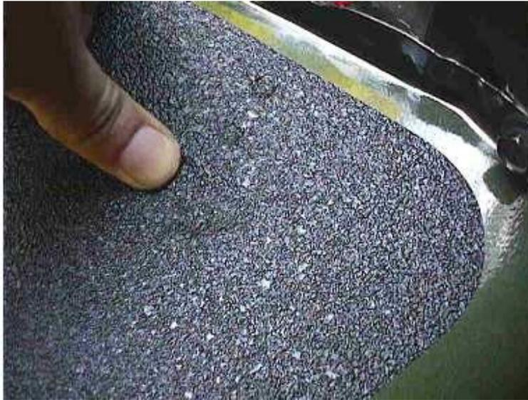
Press a Philips Head screwdriver into each indentation to open up the five (5) holes in the top of the fender needed to mount the latch and bumper.
