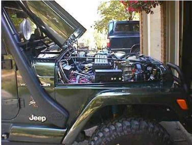
Remove your Hood Latches by unscrewing the 15mm (TJ) retaining nut underneath the fender.
