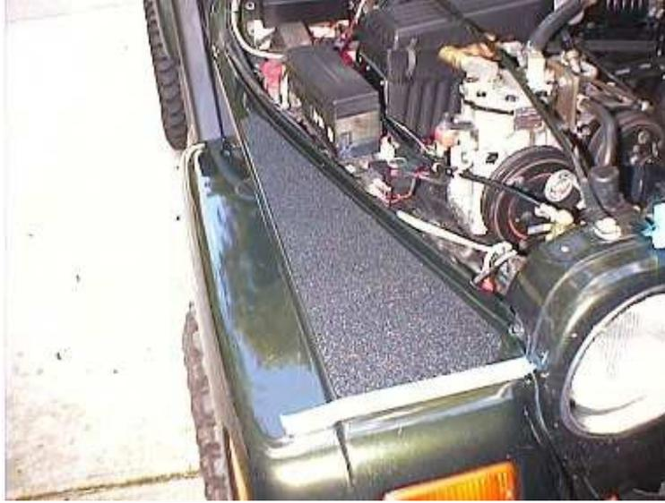
When you are satisfied with the alignment and installation, use a clean dry paper towel or the Protector Backing Paper and **thoroughly rub down the entire Protector** to finish adhesion.
