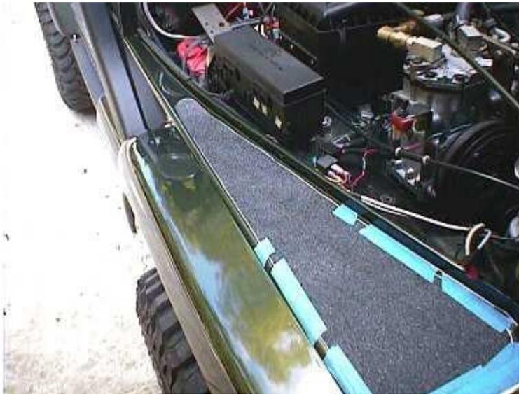
Carefully peel the adhesive backing paper off the untaped area of the Protector;
