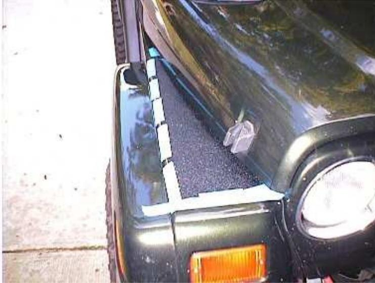
Carefully remove the masking tape **ONLY on the rear half** of the Protector. Leave the front half securely taped in place. (This will keep the Protector properly located where you want it.)
