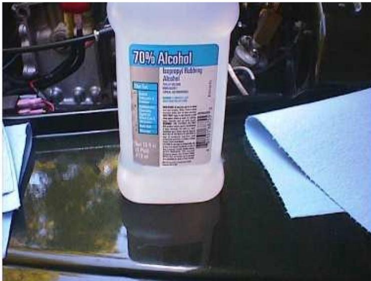
Clean each fender top one more time (fourth time). This time dry the alcohol off with a clean dry paper towel. If you see any dirt/wax film streaks while doing this repeat the cleaning process until spotless.
