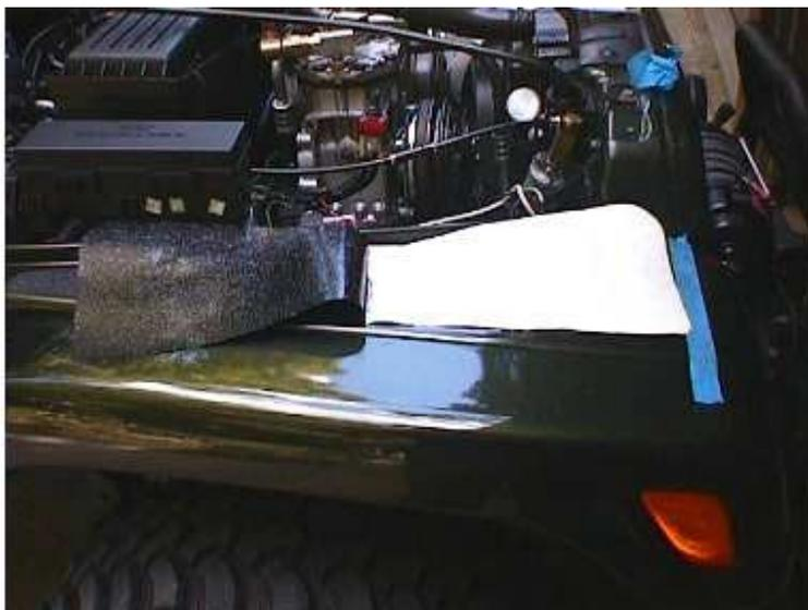
Continue to lay the front half of the Protector down onto the fender. **DO NOT rub down yet.** If the location is off you can lift the protector and re-align it.
